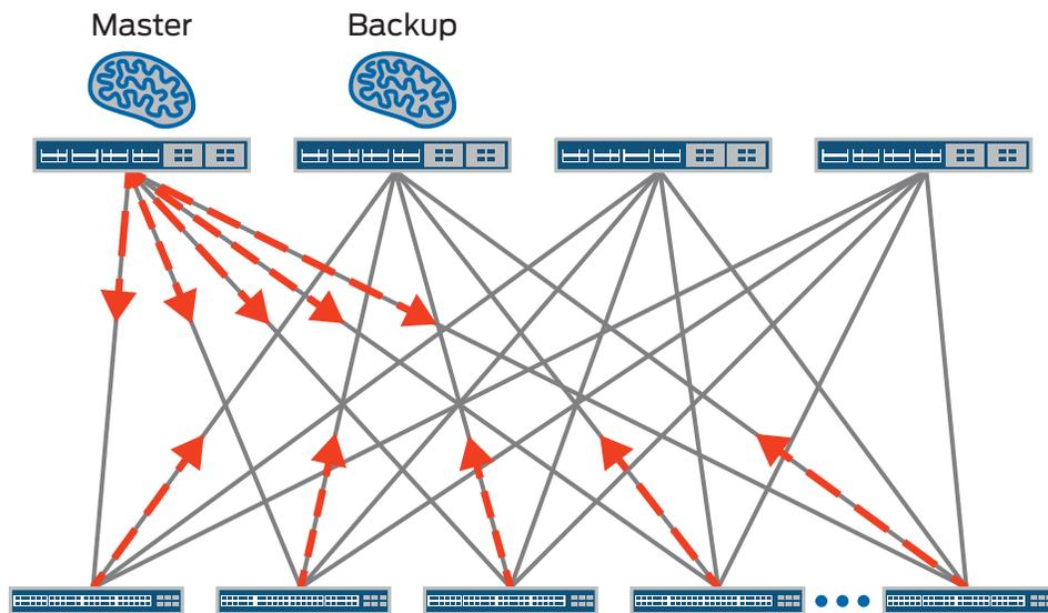
Figure 4: Virtual Chassis Fabric integrated control plane
