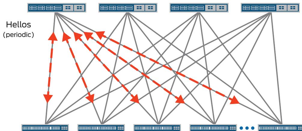
Figure 3: Autodiscovery with Virtual Chassis Fabric technology
